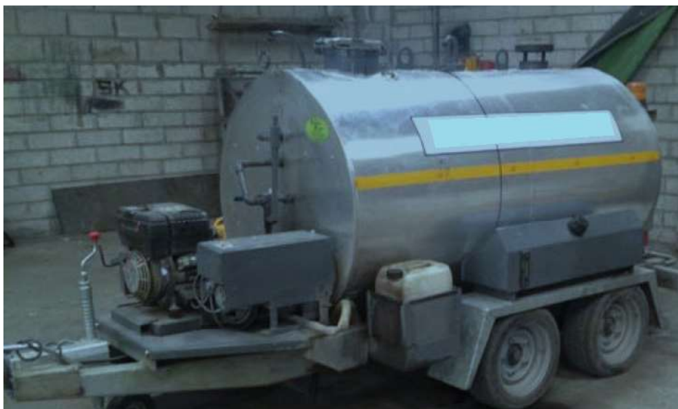
Figure 3-16: Towable Sprayer for Temporary Reinstatement
